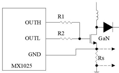
To prevent this, a common-mode choke can be used for IN+ and IN-, respectively. Resistors can also add to the signal output line before MX1025D depending on the input signal pulse width to provide additional RC filtering as shown in the following figure.
