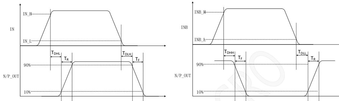
Note: OUT is tied to VDD from a small resistor
