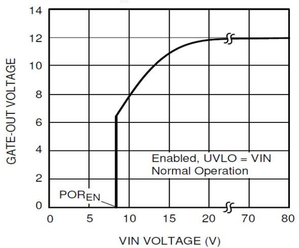
GATE Pin Voltage vs VIN
