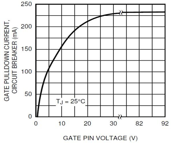
GATE Pulldown Current, Circuit Breaker vs GATE Voltage
