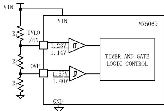
The undervoltage lockout (UVLO) and overvoltage trip point are adjusted using an external voltage divider network of  $R_1$ ,
