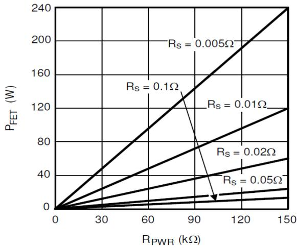
MOSFET Power Dissipation Limit vs RILIM and RS
