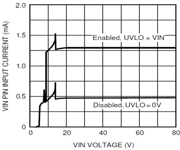
VIN Pin Input Current vs VIN
