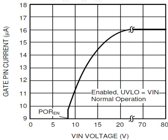
GATE Pin Source Current vs VIN
