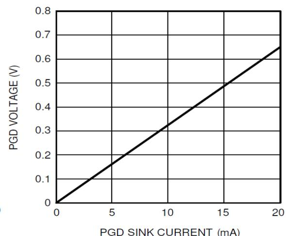
PGD Pin Low Voltage vs Sink Current
