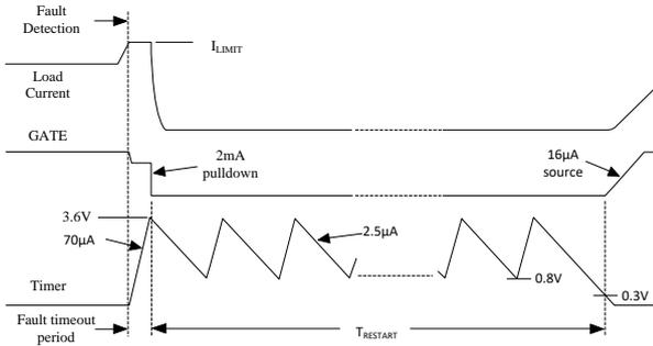
The fault timer runs when the hot swap is in power limit or current limit, which is the case during start up. Thus the timer has to be sized large enough to prevent a time out during start up. If the part starts directly into current limit the maximum start time can be computed with Equation9.
