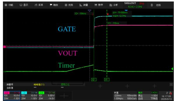
Start timing with output capacitor 1000uF
